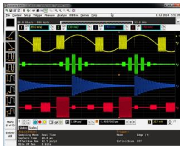
Figure 7. Four different pulsed signals up to 25 GHz.
