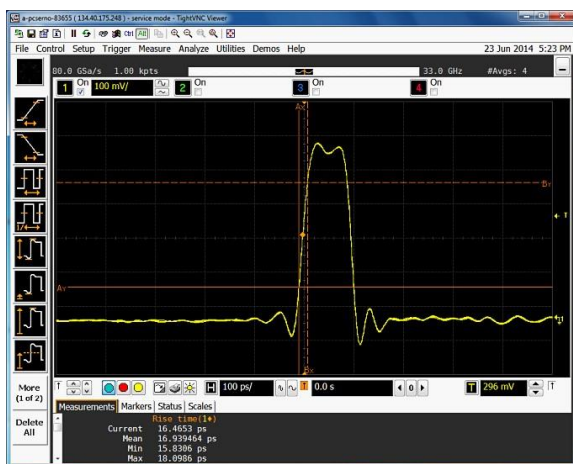
Figure 6. 100 ps pulse with 17 ps risetime.
