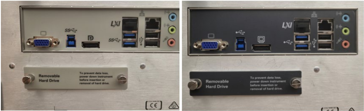
Figure 4. Motherboard Options: M900 (left) and M910 (right)
